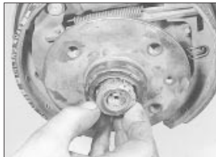
10.6a Fit the outer bearing race . . .
